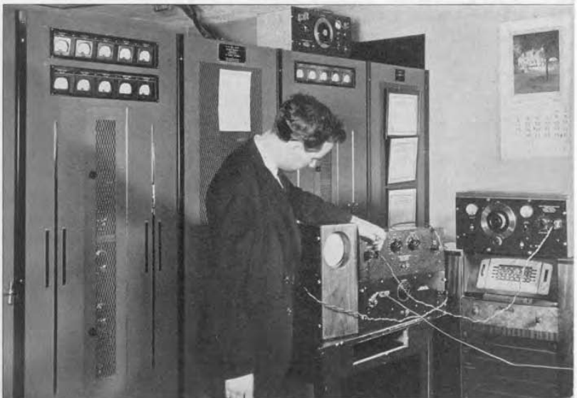
FIGURE 1. The author with the equipment used for making the tests. In the background is the frequency-modulated relay transmitter of the Yankee Network.
