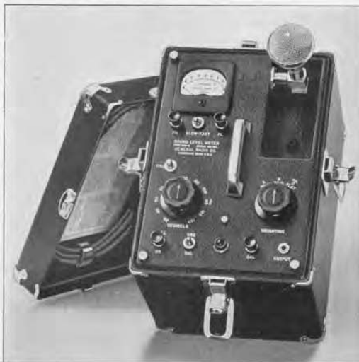
FIGURE 1. View of the Type 759-B Sound-Level Meter with cover removed.
