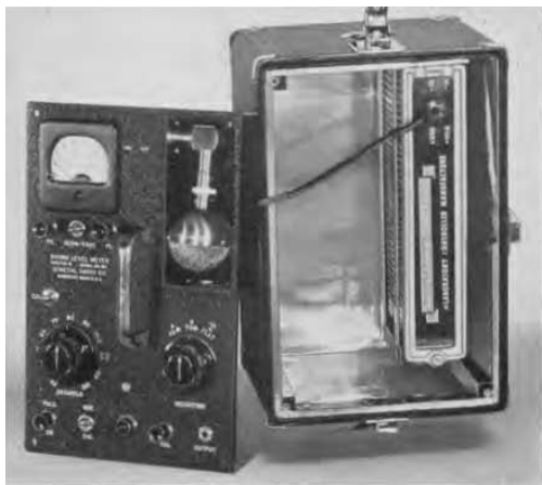
FIGURE 2. The power supply for the sound-level meter is a single block battery which mounts inside the cabinet. Connections are made with a plug as shown.
